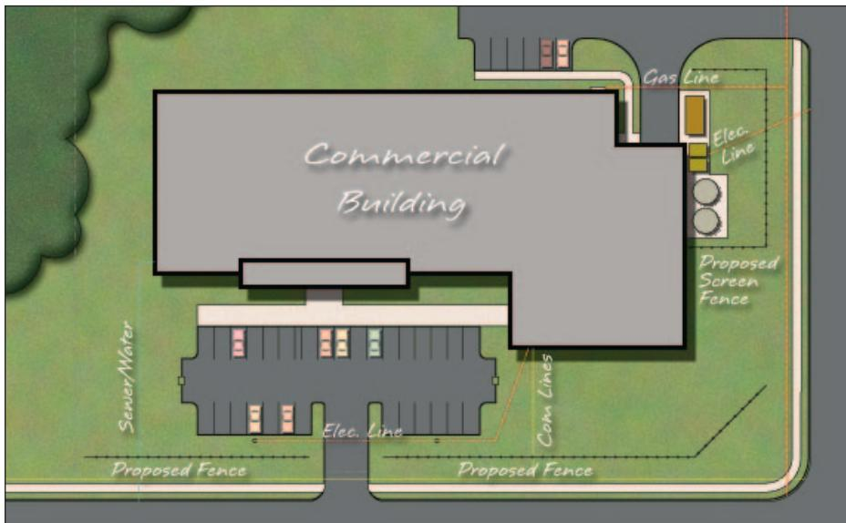
A detailed site plan drawn to scale will help foresee design and construction challenges and provide an accurate reference for estimating.
