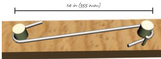
Install stirrups as described on page 46 prior to vibrating. This will ensure a quality bond beam for maximum stability.
