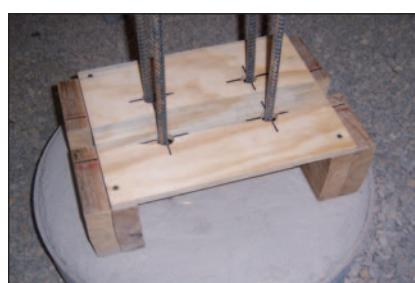
Figure 3: Optional Rebar Alignment Jig
