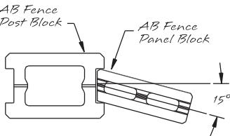
Cut And Rotate The AB Fence Panel Block A Maximum Of 15.0° To Create Tighter Radii.
