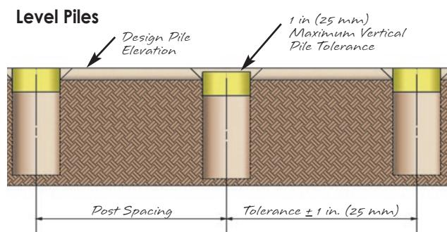
Figure 9: Pile Hole Cross Section
