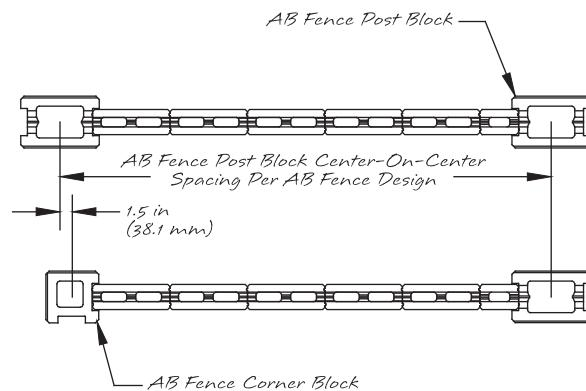
For each corner location the center-on-center spacing needs to be reduced by 1.5 in (38 mm). If AB Fence Corner Blocks are used on both ends of a panel, the center-on-center spacing is 3 in (75 mm) shorter than if two AB Fence Post Blocks are used. See the AB Fence Tech Sheet #2005 at [allanblock.com](http://allanblock.com) for additional information.
