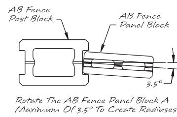
Rotate The AB Fence Panel Block A Maximum Of 3.5° To Create Radii.
