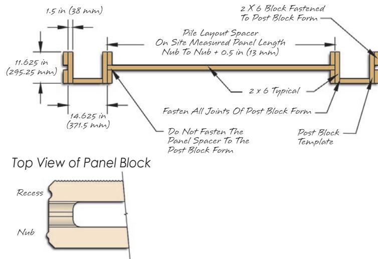
Figure 2: Post Block Template with Pile Steel Placement
