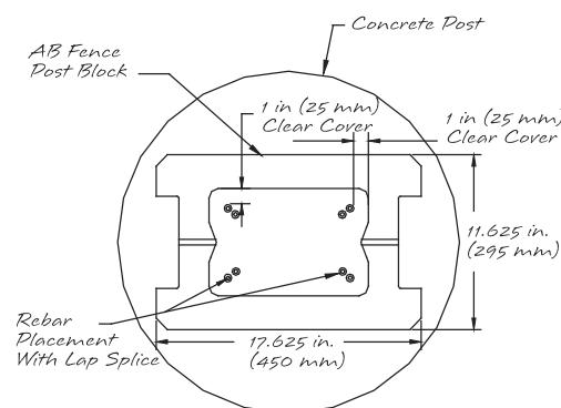
**Note:** The AB Fence uses two different types of concrete during construction. The piles and AB Fence Post Blocks use concrete with gravel and sand size aggregate. This type of concrete is generally available from concrete plants and used in most types of construction. However, the bond beams require what is referred to as a fine mix concrete grout. This mixture of concrete uses only sand as the aggregate, which makes it ideal for filling the smaller cores of the AB Fence Panel Block.
